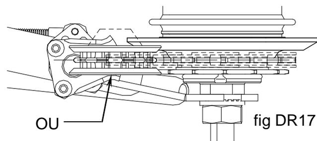
**Cable adjustment** should seldom be necessary, as the trigger moves the cable twice as far as the movement of the chain-pusher (an over-ride spring *inside* the dogleg DL absorbs this movement).
